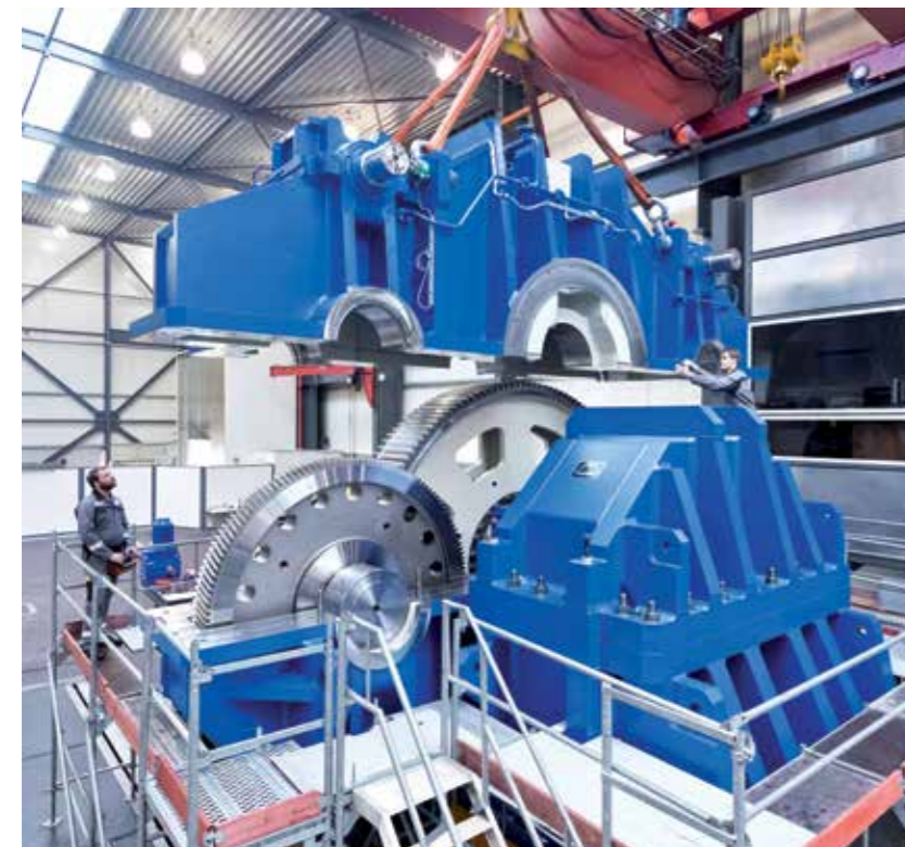
Cutter Gear unit type: CDSHII-4800 Power: 2 x 4,250 kW Speed: 1,000/30 rpm
